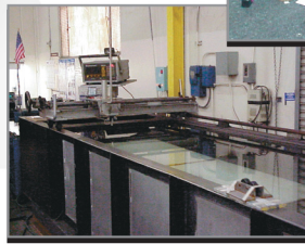
Ultrasonic Inspection tank for inspecting forge bar stock and forged parts.
