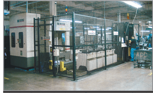
4-axis Horizontal CNC Center with 9 pallet cell
