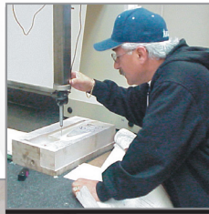
Ultrasonic Inspection tank for inspecting forge bar stock and forged parts.
